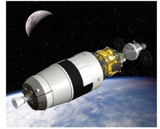
Concept image of the Ares V Earth departure stage in orbit, shown with the Orion capsule docked with the Altair lander (NASA MSFC)
