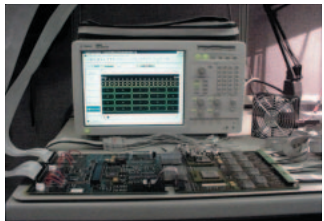
Figure 3 – Laboratory set-up using the Agilent 1680A benchtop logic analyzer
