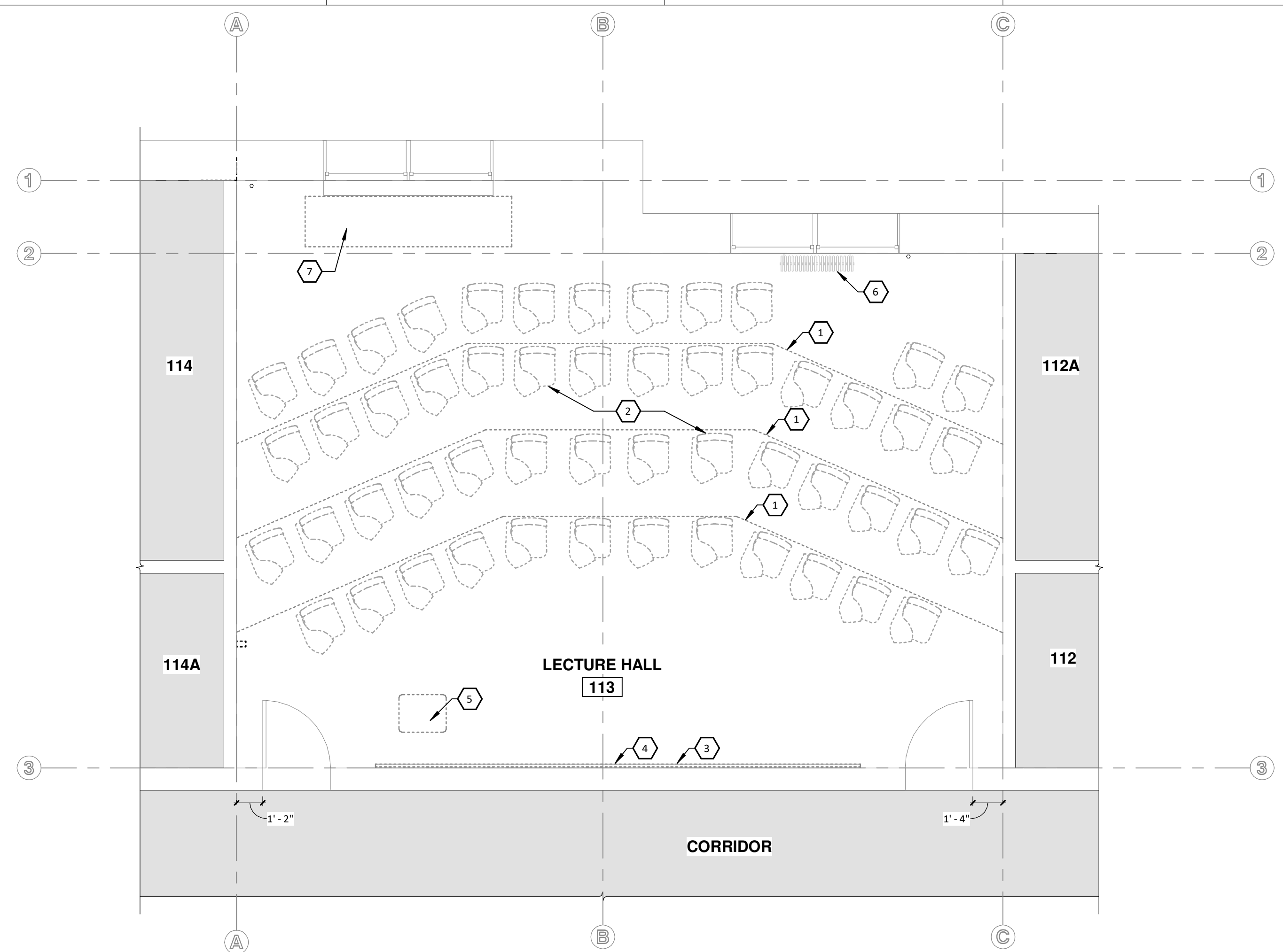
1 DEMO FLOOR PLAN 1/4" = 1'-0" APPROXIMATE OCCUPANCY: 52 (15.9 S.F./STUDENT)
