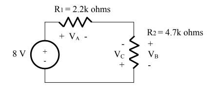
**P2.** Using the voltages you measured in P1, show two examples of Kirchhoff's voltage law: one expression using your measurements for  $V_A$ ,  $V_B$ , and the 8 V power supply, and another expression using your measurements for  $V_A$ ,  $V_C$ , and the 8 V power supply. Explain the reason for any discrepancy in your measurements.
