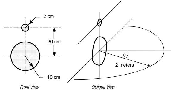
Each driver is modeled as a baffled piston radiator (far field case). The drivers are operated at f = 4 kHz into air at 20°C.
