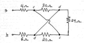
Notice that the points labeled c are the same node and that the points labeled d are another node. Thus, the 30- $\Omega$ , 24- $\Omega$ , and 20- $\Omega$  resistors are in parallel because they are each connected between nodes c and d. The equivalent resistance is 18  $\Omega$ .
