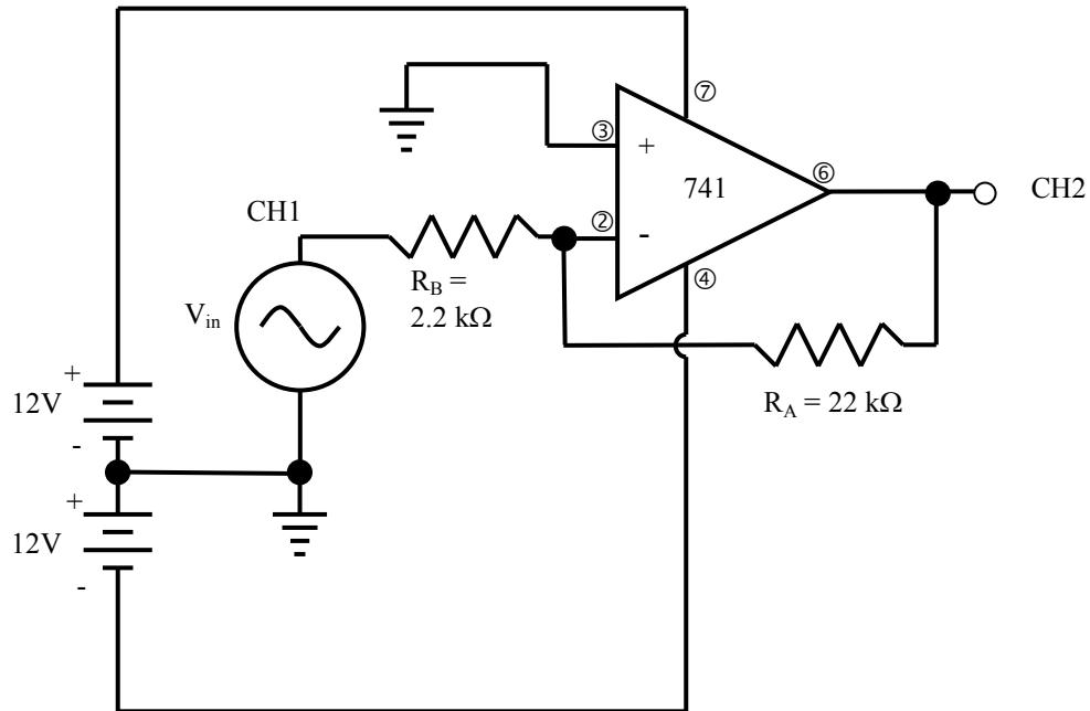
Inverting amplifier configuration:
